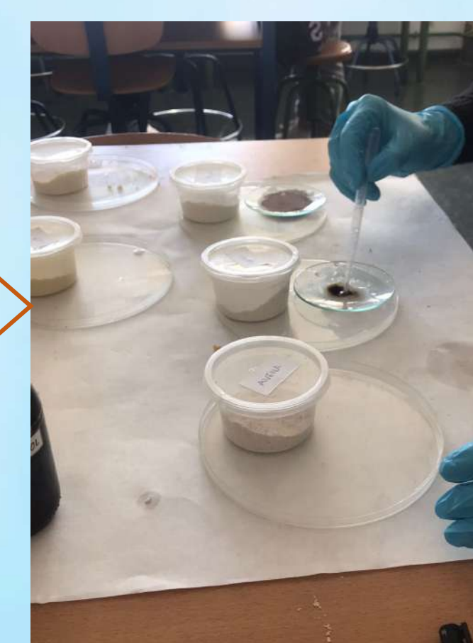
Picture 3: Analytical determination to check the loss of starch with washing
