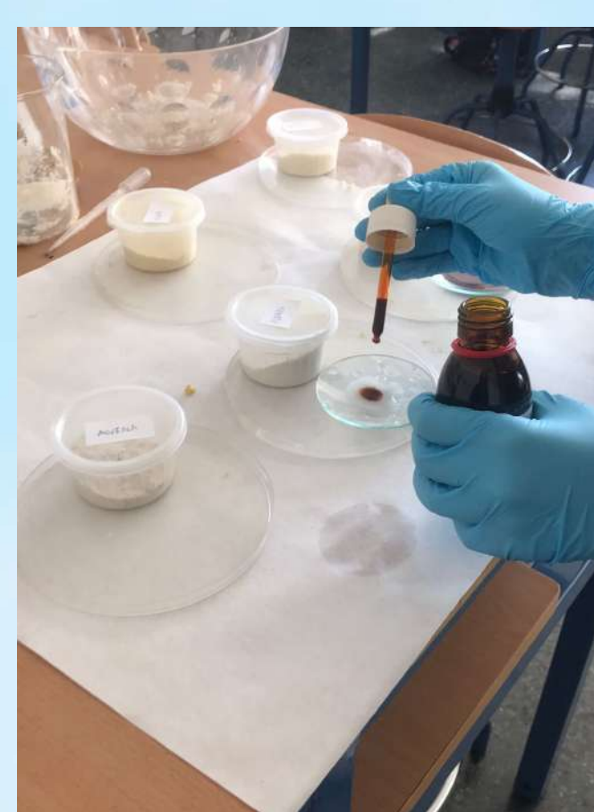
Picture 2: Analytical determination to check the loss of starch with washing
