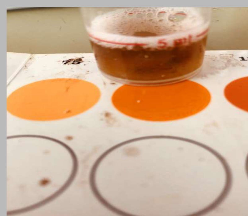
Figure 5. Nitrate test result in standing water.
