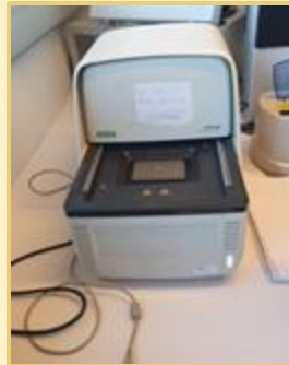
qPCR MACHINE. Thermocycler.
