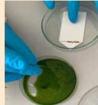
Fig. 24 Placing the pigment onto the chromatography paper
